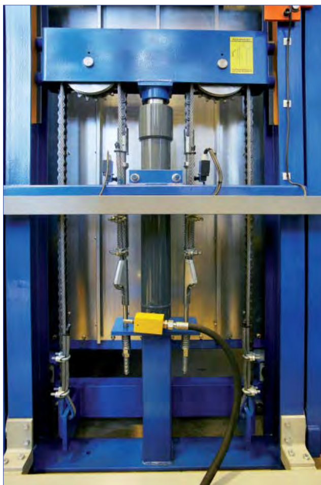
Figure 7. Rear view of the lower guiding structure, pre-assembled.
