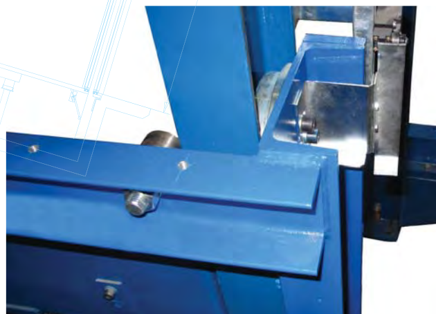
Figure 6. Lateral Guiding, 4 bearings per frame.
