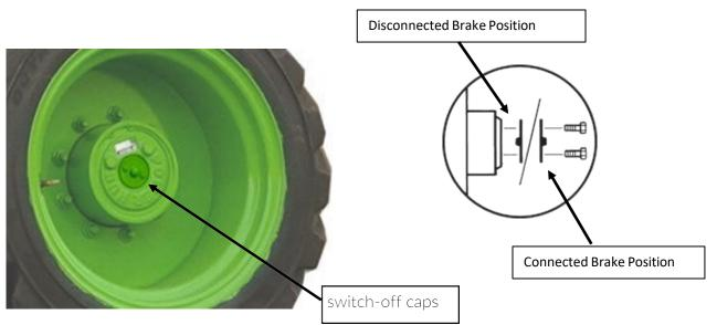
Steering the wheels when the vehicle is towed
