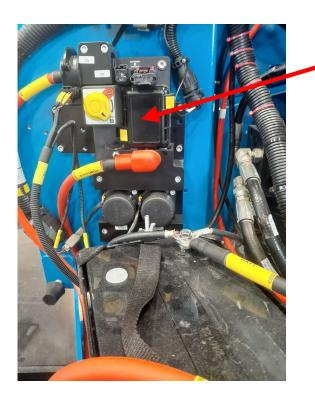
Fuses have been removed for transport. These are located under the lid, see picture
