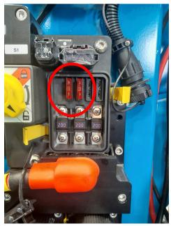
In transport mode, fuses are placed in the two free slots
